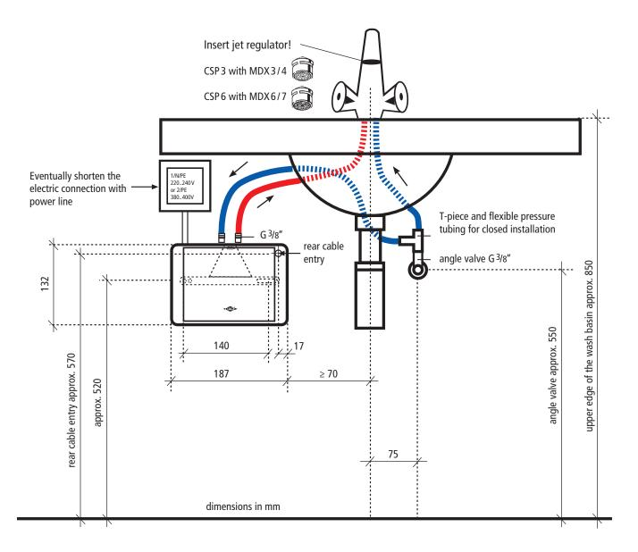
Example of installation with closed outlet tap.
