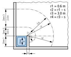
The instantaneous water heater for the type M../BGS shower is protected by an IP 25 housing and may be installed in protective zone 1 according to VDE 0100 Part 701.
